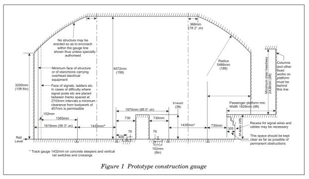
The horizontal distances between prototype tracks and adjacent structures are increased for curved track to allow for the throw-over of long vehicles. Radius of Curve in metres - all horizontal distances increased by
