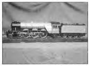
Photo 1.14 A Flying Scotsman by A.W. Mills of Cheltenham. This is internally fired with meths burners and has been overhauled by Clarry Edwards. (Photo R. Fielding).
